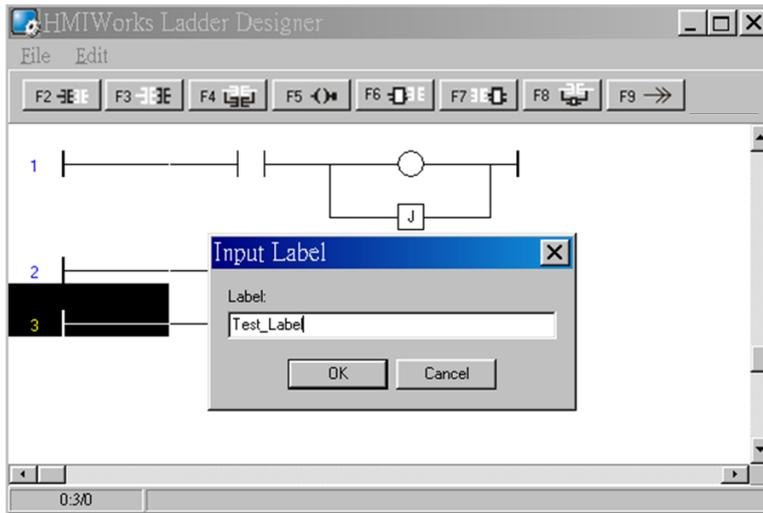
4. Double click on the Jump of the first rung to associate with the label of the third rung.
