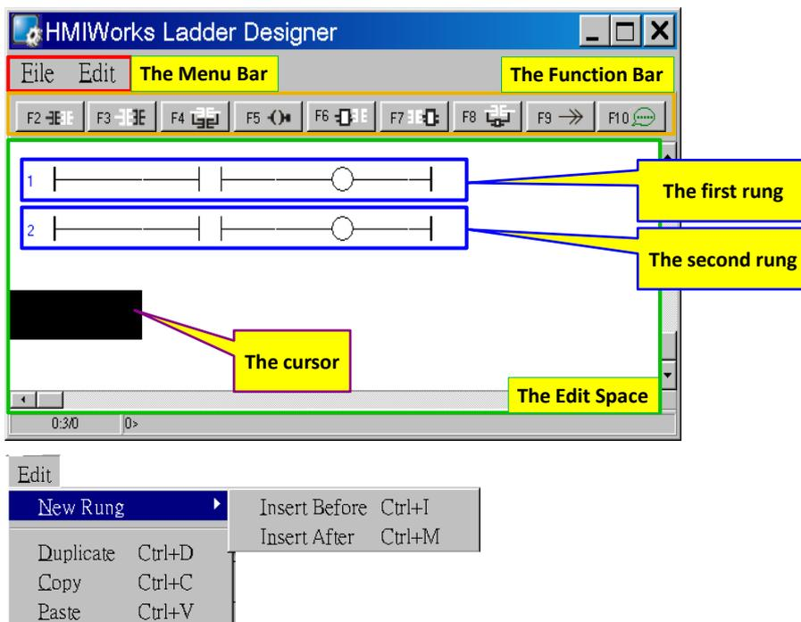
Mainly, a **Ladder Designer** consists of three parts, the menu bar, the function bar, and the edit space. The highlighted rectangle area is the cursor.
