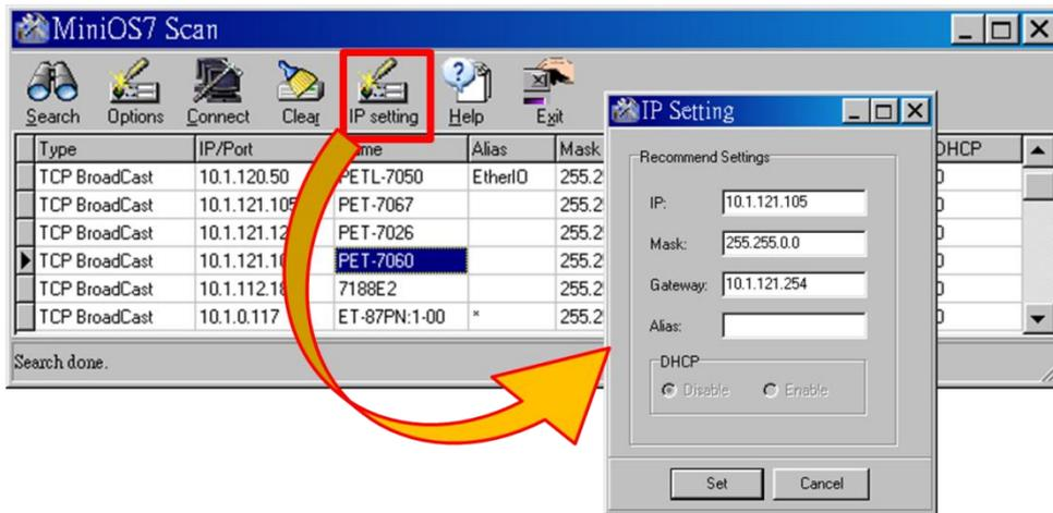
Finally, connect to the PET-7060 module and configure it by a browser.
