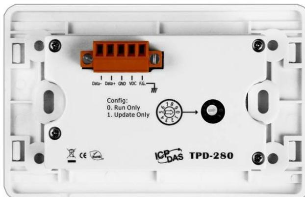
On the back panel of the TPD-280 device, configuration modes can be found. Use the rotary switch to set the configuration mode.
