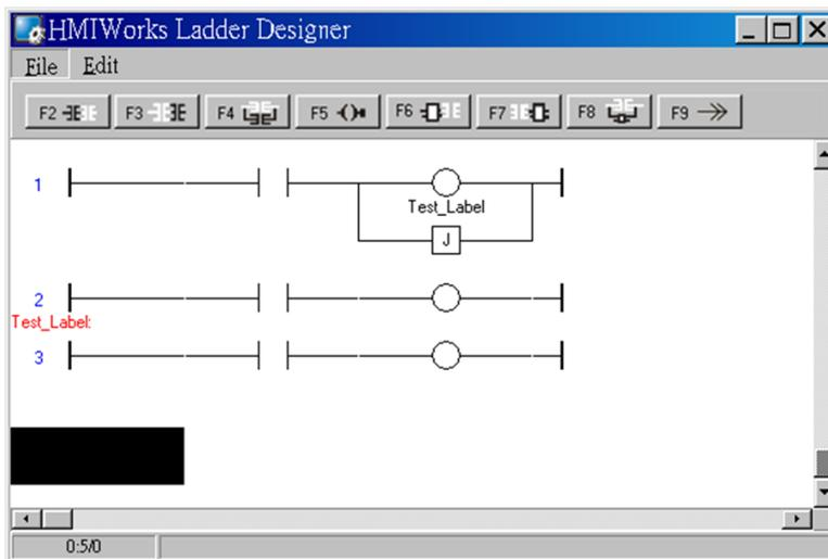
5. When running the ladder logic, set the coil output of the first rung to high, skip the second rung and jump to the third rung if the contact input of the first rung is closed.
