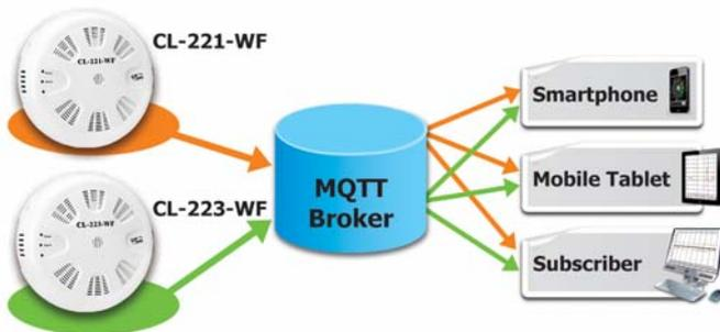
Real-time data from the CL-200-WF series can be accessed from anywhere and at any time using the WF-IIOT-Utility and iOS App.
