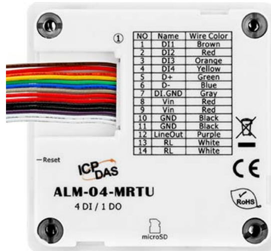
Figure 2-6: Wire color & function
