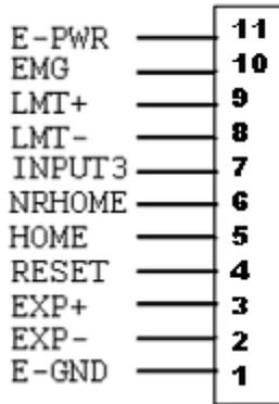
Fig. B4-6 Pin definition for CN1 & CN2
