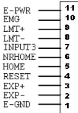
Fig B3-6 Pin definition for CN1 & CN2
