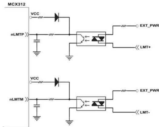
Fig. 2.11 Limit switch signal circuit
