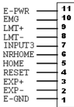
Fig. B1-6 Pin definition for CN1 & CN2
