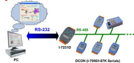
I-7231D main unit can connect to the DCON(I-7K/I-87K) IO modules to create a customized CANopen slave device and application. In order to allow user to easy apply the device on the network, ICP DAS also provides the I-7231D Utility tool to configure the IO connection path, assembly and application objects information and create the EDS file of the device.
