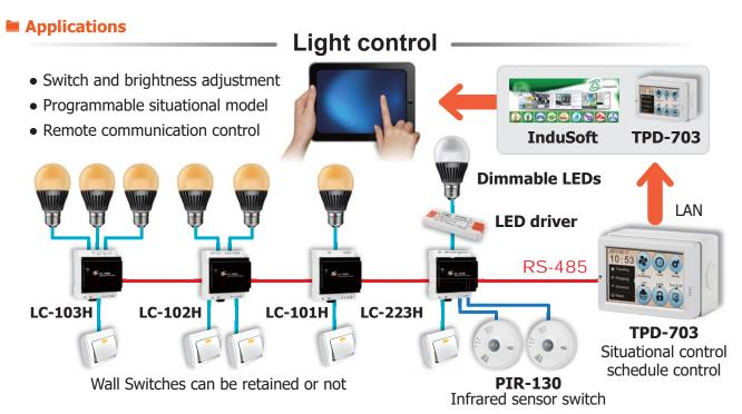
(For example: when 10 lamps are normally connected, the current is 2.2A. When the reading is less than 2.2A, it can be judged that there is a lamp failure and it needs to be repaired)
