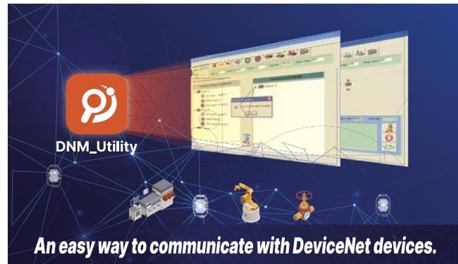
This utility supports to search all devices and specific devices in the network and can configure the I/O connection of the devices by searching devices or manual setting. It can easily to access the I/O data of all the slave devices.
