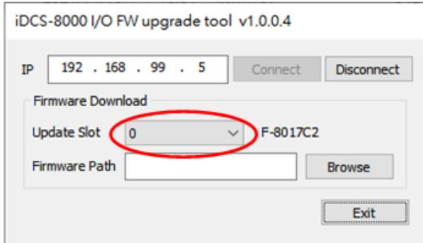
Step6: Select the file (.fw) to start updating the firmware of the I/O Module.
