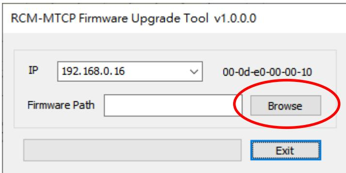
**Step10:** Update the RCM-MTCP firmware
