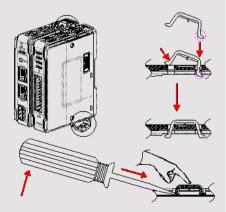
Rail mounting: DIN rail 35mm.
